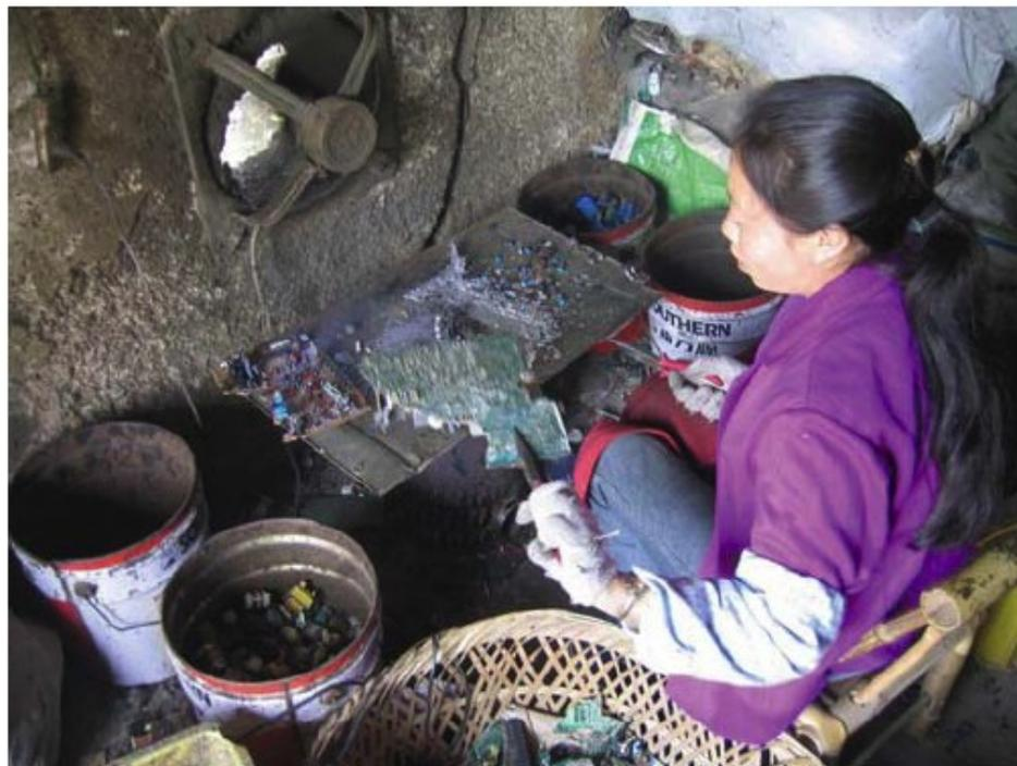
Figure 3. Circuit board baking.
